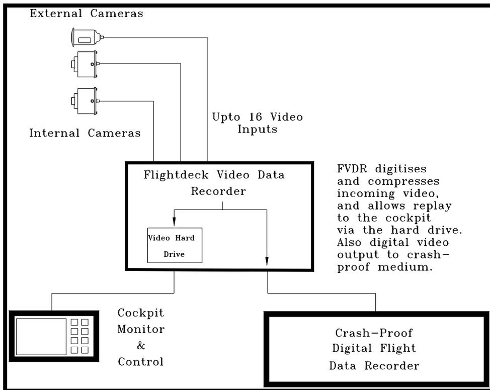
**Figure 2 - Crash Proof Flightdeck Video Data Recorder**
